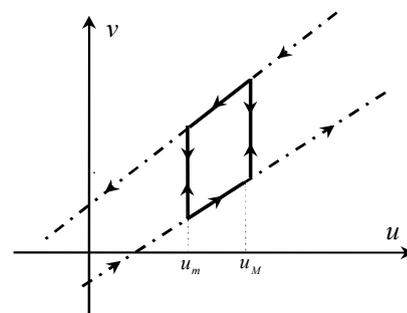
Fig.6b. Example of obtained backlash cycle for a small working interval.
