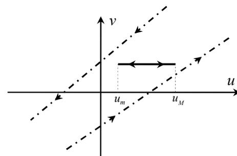
Fig.6a. The Backlash cycle reduces to a horizontal segment.
