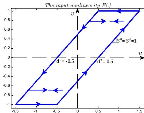
Fig.9. The Backlash operators considered in simulation.
