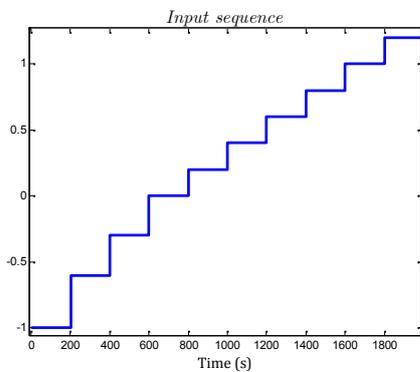
Fig.10. Input signal used for the identification of the system nonlinearities.
