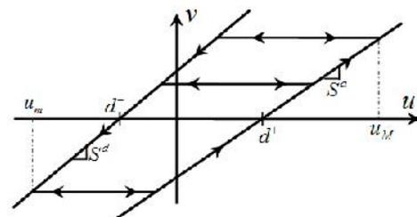
Fig.2. Backlash bordered by straight lines.
