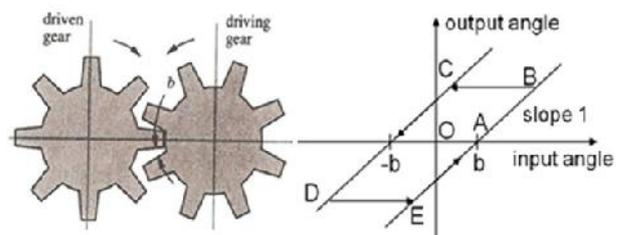
Fig.4. The backlash occurs as result of the gaps between a pair of mating gears.
