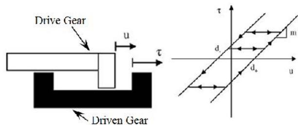
Fig.3. Example of Backlash nonlinearity occurring in mechanical systems.
