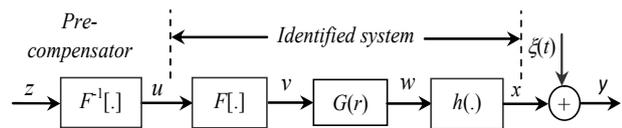
Fig.8. The system to be identified augmented with pre-compensator.
