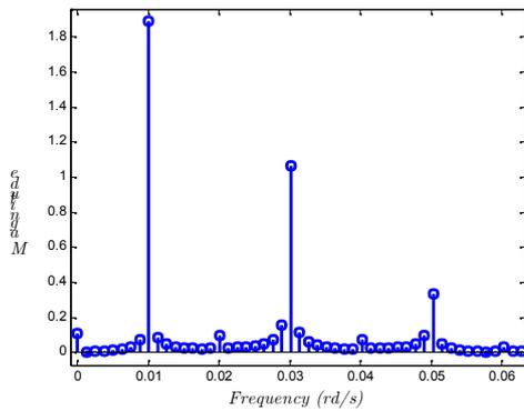
Fig.16a. Fourier transform modulus of  $\hat{x}_N(t)$ .
