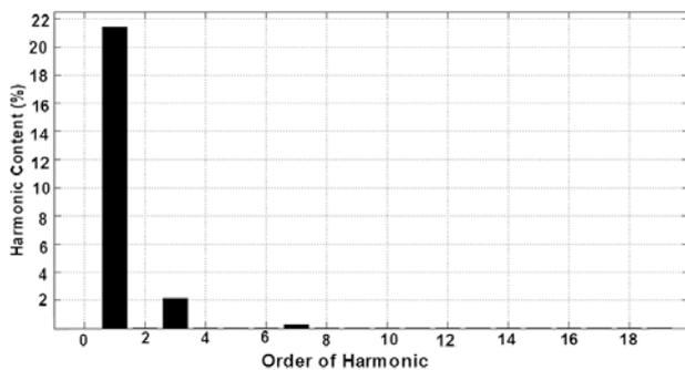
Fig. 8 Current harmonics under distorted balanced grid voltages during constant power operation.
