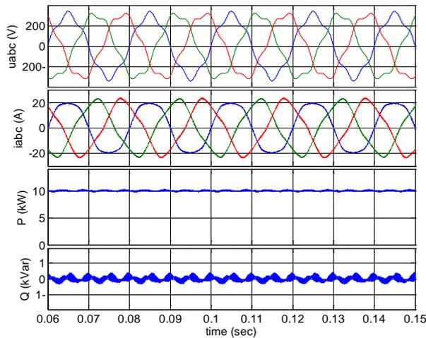
Fig. 7 System performance under balanced grid voltages superimposed by a fifth order harmonic component.
