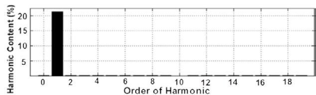
Fig11 Current harmonics under unbalanced grid voltages during sinusoidal current operation.
