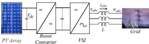
Fig.1 PV grid connected system.
