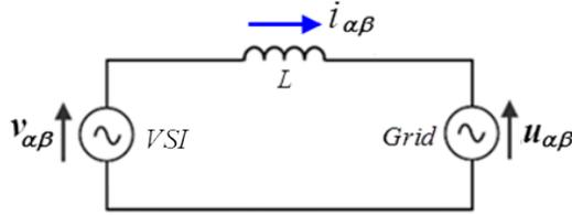
Fig. 4 System model in stationary reference frame.
