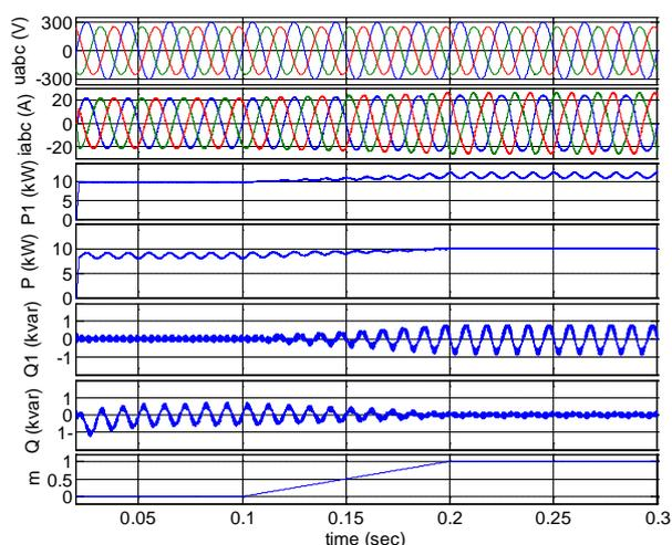
Fig. 14 Switching between constant power control and sinusoidal current control. Plots from top to bottom: unbalanced grid voltages, grid currents, virtual  $P_1$ , actual  $P$ , virtual  $Q_1$ , actual  $Q$  and adaptive factor  $m$ .
