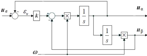
Fig.3 Adaptive filter based on the SOGI.
