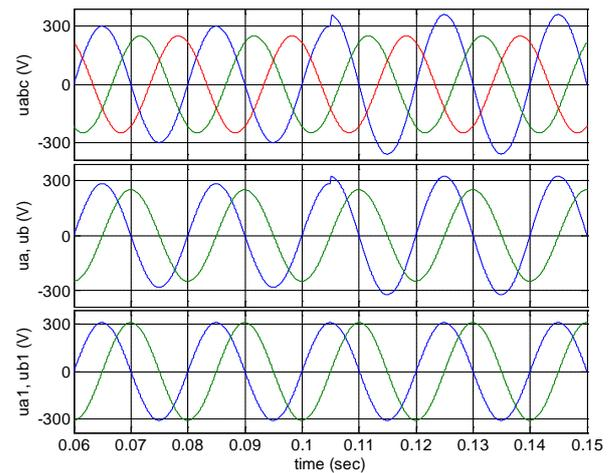
Fig. 9 Generating virtual grid voltage in  $\alpha\beta$  frame under unbalanced grid voltages during step change in phase-a voltage, from top to bottom, 3-phase grid voltages, actual  $u_\alpha, u_\beta$  and virtual voltages  $u_{\alpha 1}, u_{\beta 1}$ .
