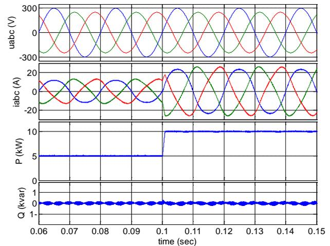
Fig.5 Constant power operation, from top to bottom: unbalanced grid voltages, grid currents, actual power (P), and actual reactive power (Q).
