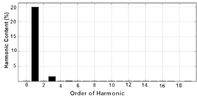
Fig. 6 Current harmonics under unbalanced grid voltages and constant power operation.
