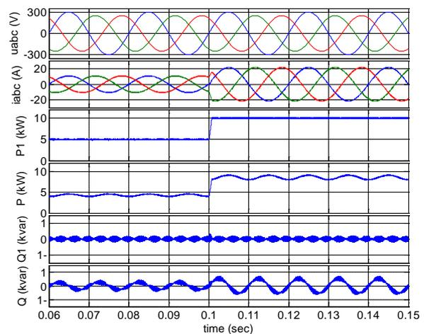
Fig. 10 Sinusoidal current operation, from top to bottom: Unbalanced grid voltages, grid currents, virtual  $P_1$ , actual  $P$ , virtual  $Q_1$ , and actual  $Q$ .
