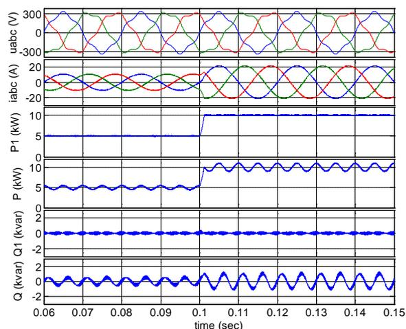
Fig. 12 System performance under balanced grid voltages superimposed by a fifth order harmonic component (sinusoidal current operations).
