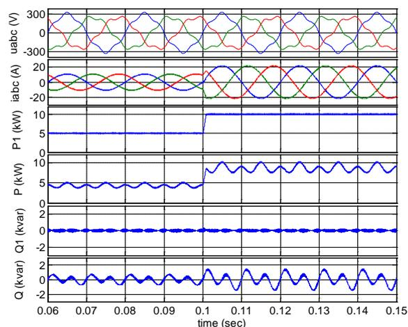
Fig. 13 System performance under unbalanced grid voltages superimposed by a fifth order harmonic component (sinusoidal current operations).
