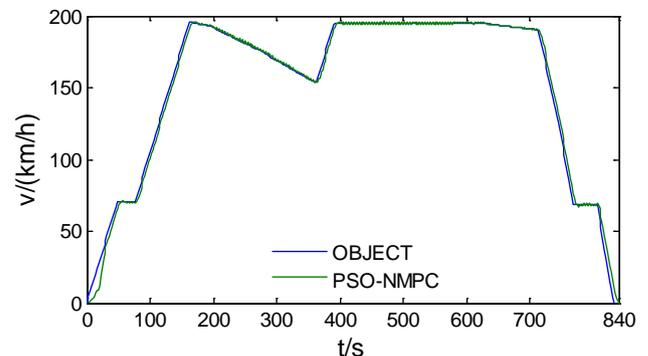
Fig.8 PSO-NMPC follow the V-t curve
