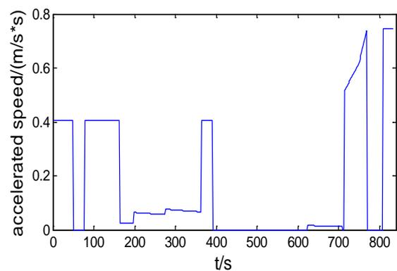
Figure 5 The acceleration curve of target curve from the figure that in the whole operation process the acceleration is less than  $1\text{m/s}^2$ , so that the comfort for passengers is ensured.
