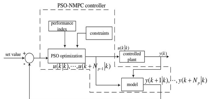
Figure7 PSO-NMPC Control structure
