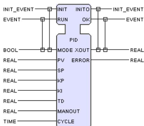
Fig. 7. The PID composite function block
