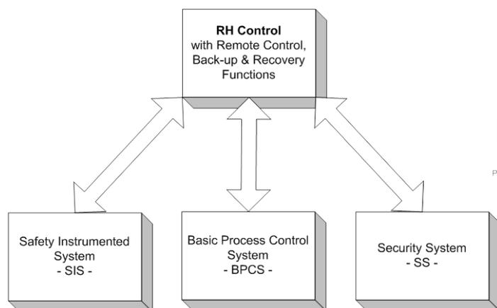
Fig. 4 Functional Architecture incorporating Risk and hazard control
