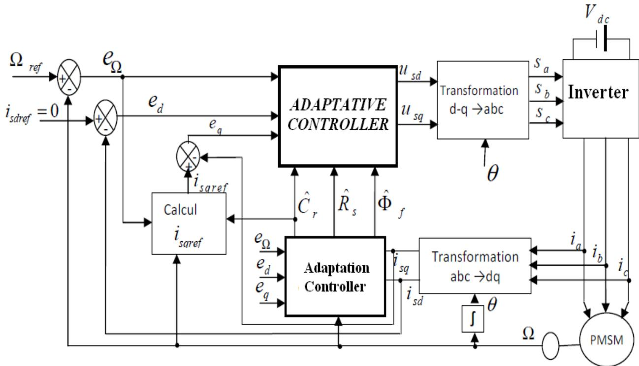
Fig.6: System configuration of adaptive Backstepping Control
