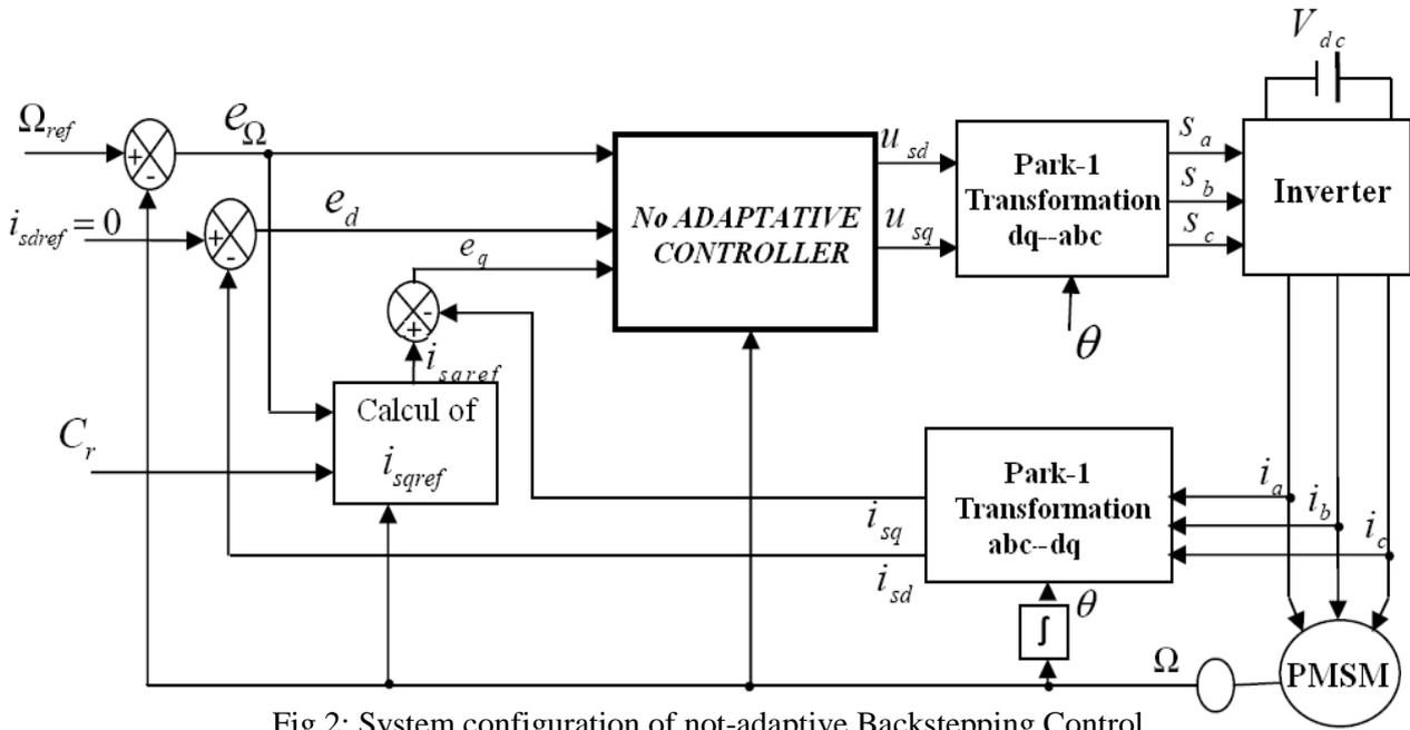
Fig.2: System configuration of not-adaptive Backstepping Control
