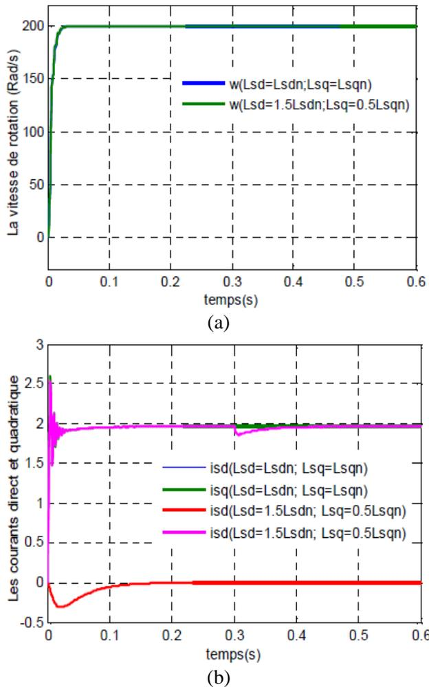
Fig.11: Test performance of the adaptive controller following a change in  $L_{sd}$  and  $L_{sq}$
