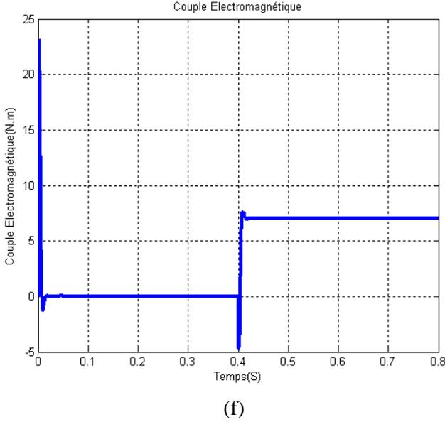
Fig.5: (a) Speed response trajectory, (b) Error Speed response, (c) abc Axis Stator Current, (d) dq Axis Stator Current, (e) d-q Axis Stator Flux, (f) Electromagnetic Torque  $C_e$
