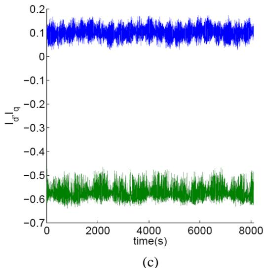
Fig.16: (a) Stator current locus for ISMC, (b) abc-axis current in the PMSM, (c) d-axis and q-axis current in the PMSM
