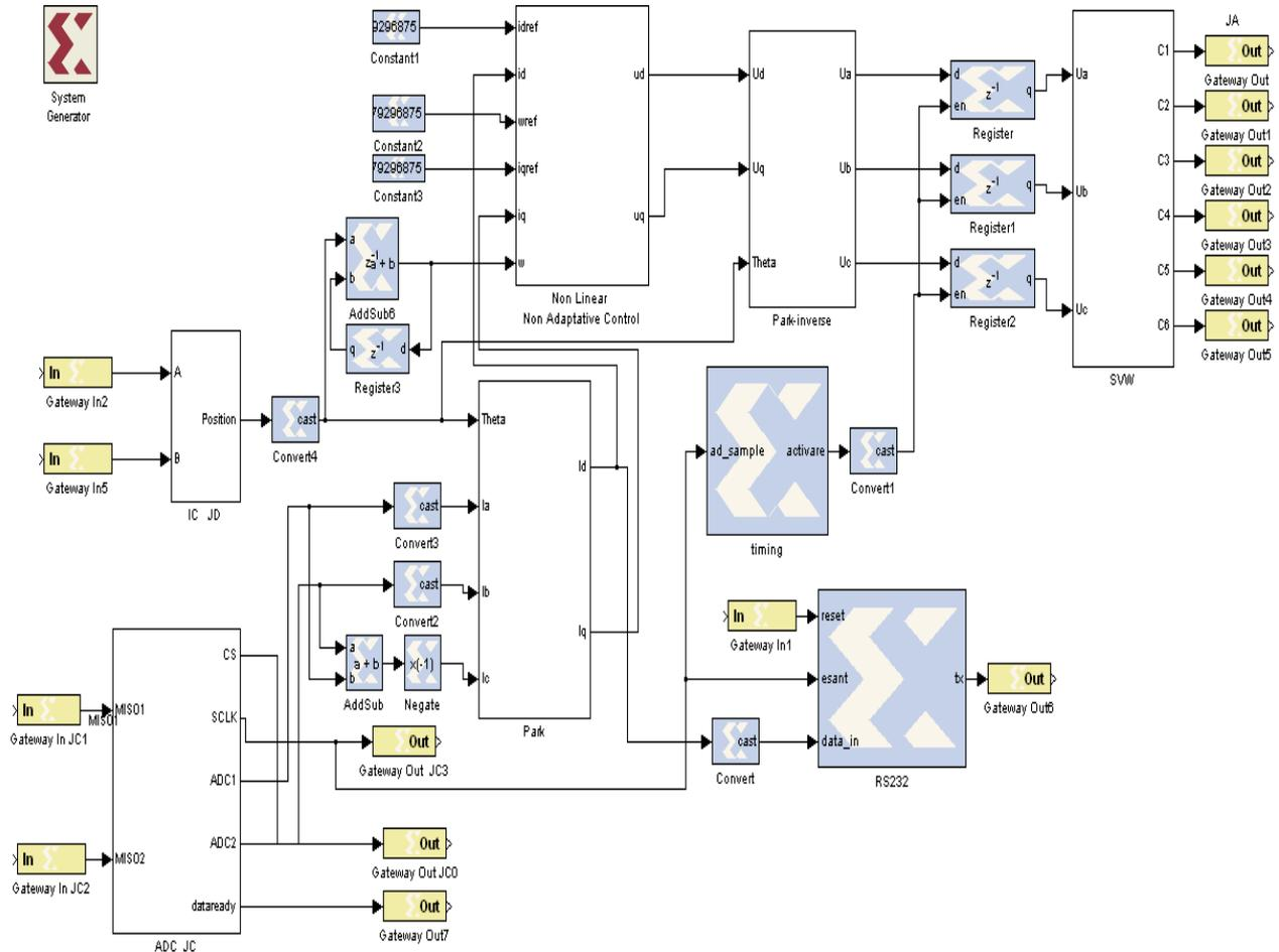
Fig.13: Functional Model for No adaptive Backstepping Controller from SYSTEM GENERATOR
