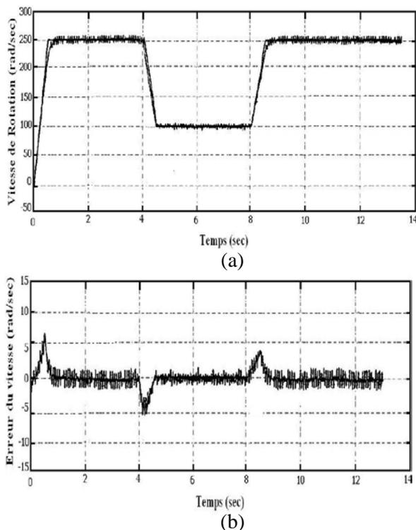
Fig.16: (a) Speed performance rotor of PMSM, (b) Error Speed performance
