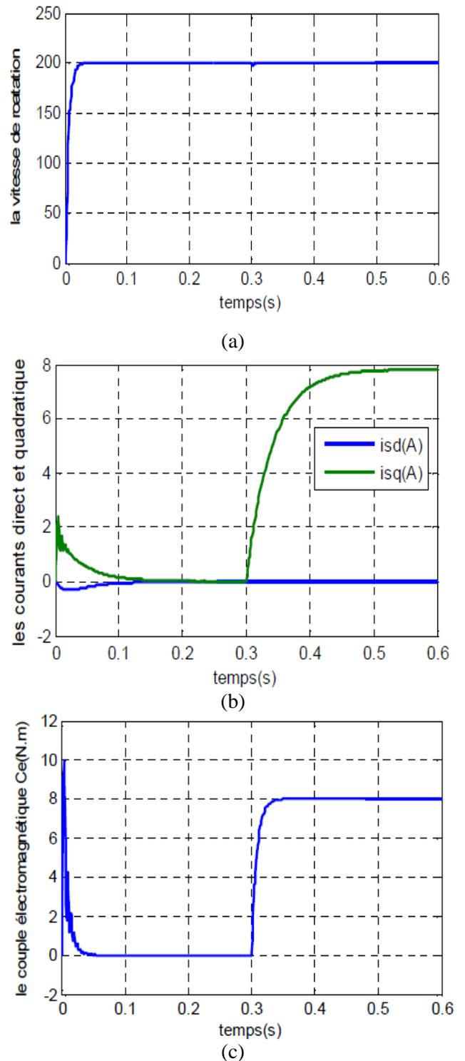
Fig.8: Test performance of the adaptive controller for rejecting disturbance torque load applied at  $t = 0.3s$ .
