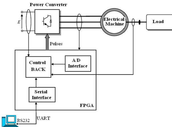
Fig.1: Architecture of the Control
