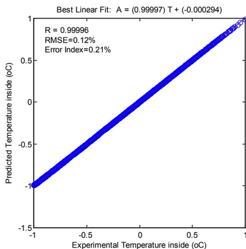
Fig. 12 The NN predictions for inside temperature vs. the actual inside temperature for model N3
