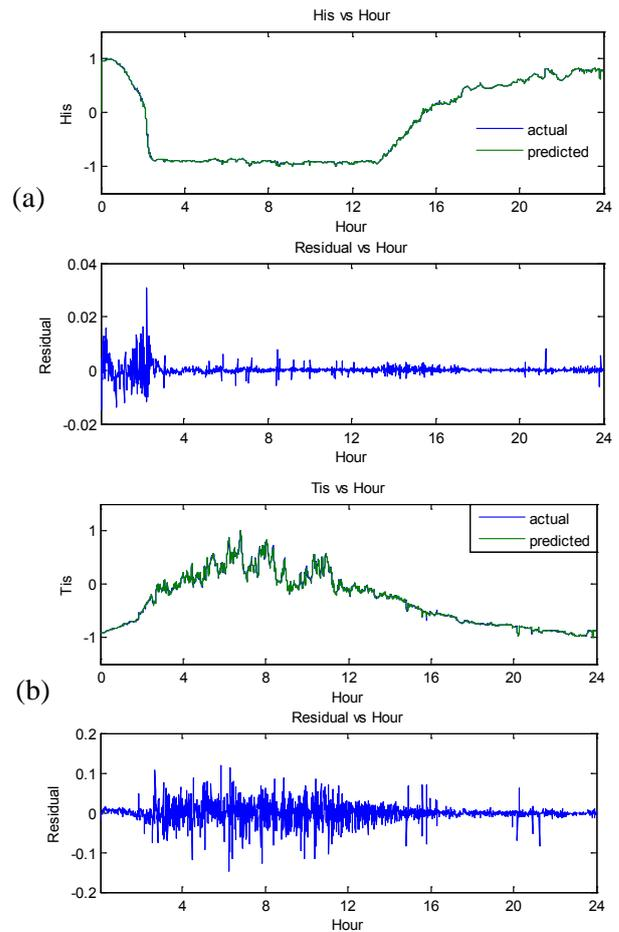
Fig. 6 The predicted and actual outputs (Humidity inside,  $H_{is}$  and Temperature inside,  $T_{is}$ ) and residual for the model 3 of ARX
