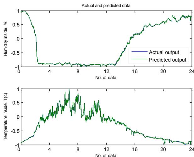
Fig. 9 The actual and predicted outputs for temperature and humidity for model N3.
