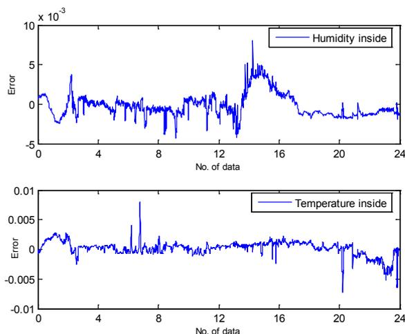
Fig. 10 Residuals of the predicted output with actual output for model N3
