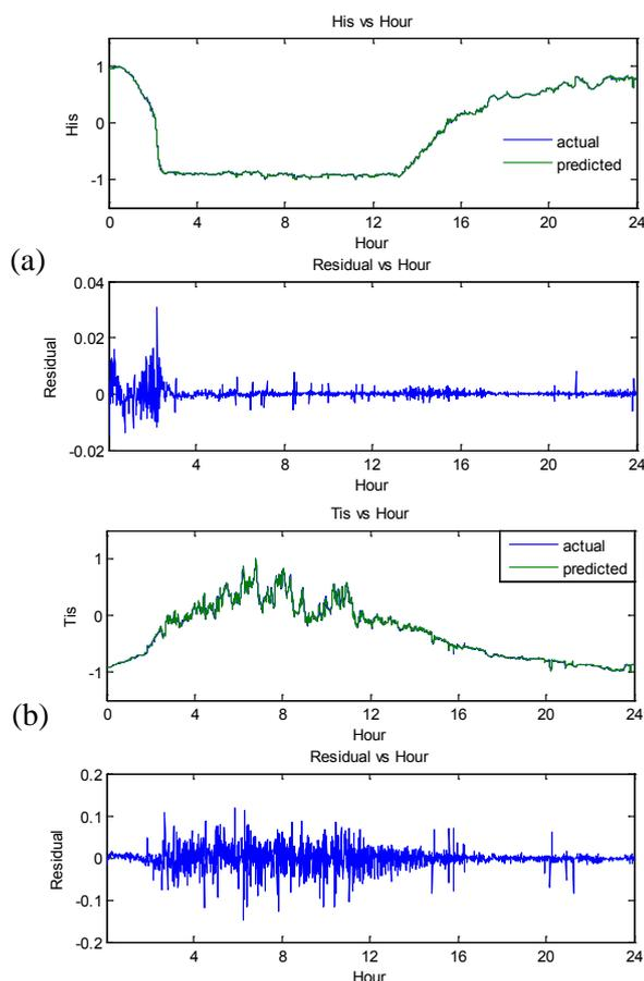
Fig. 7 The predicted and actual outputs (Humidity inside,  $H_{is}$  and Temperature inside,  $T_{is}$  ) residual for the model 3 of NARX
