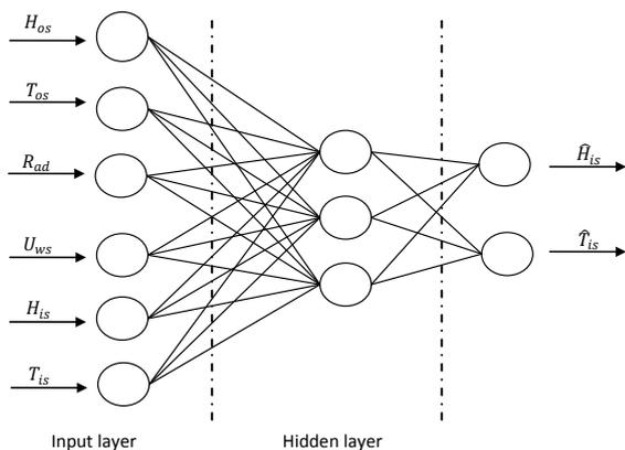
Fig. 8 The architecture of ANN model for NVTG system.
