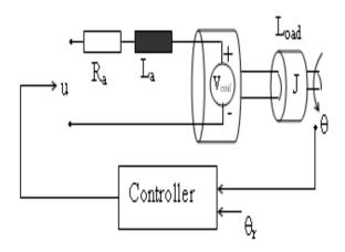
Fig.1: DC Servomotor circuit diagram
