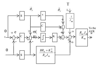
Fig. 3: Block diagram of the conventional SM controller
