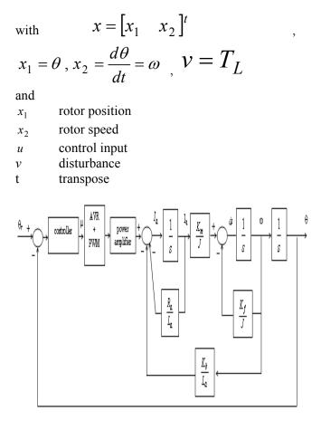
Fig. 2: Block diagram of the DC motor with AVR.
