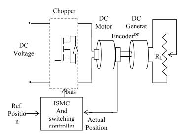
Fig. 9: DC motor drive system configuration
