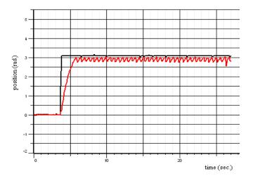
Fig. 11: Experimental time response of the SMC driven DC servo motor
