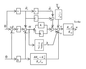
Fig. 4: Block diagram of the proposed ISM controller with switched gains
