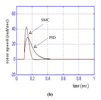
Fig. 5: Time response of the SMC and optimization tuned PID driven DC servo motor (a- Rotor Position in Rad., b- Rotor Speed in Rad/Sec.)
