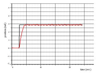
Fig. 14: Experimental time response of the PID controller driven DC servo motor with external disturbance.
