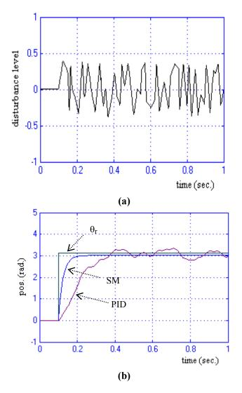
(c) Fig. 6: Time response of the proposed SMC driven DC servo motor with matched disturbance (a-Disturbance level, b- Rotor Position in Rad., c-Rotor Speed in Rad/Sec.)
