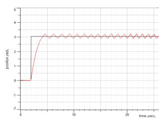
Fig. 12: Experimental time response of the ISMC driven DC servo motor
