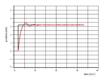
Fig. 13: Experimental time response of the ISMC with gain changed driven DC servo motor
