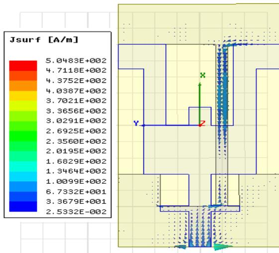
Fig. 11 Bottom View of Surface Current Density at 3.926 GHz
