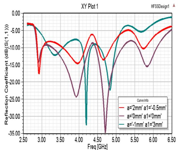
Fig. 17 Parameters *a* and *a1*
