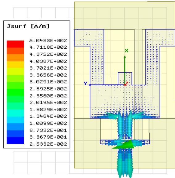
Fig. 6 Top View of Surface Current Density at 7 GHz
