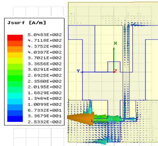
Fig. 13 Bottom View of Surface Current Density at 4.706 GHz
