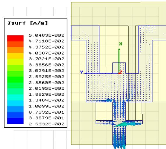
Fig. 14 Top View of Surface Current Density at 5.837 GHz
