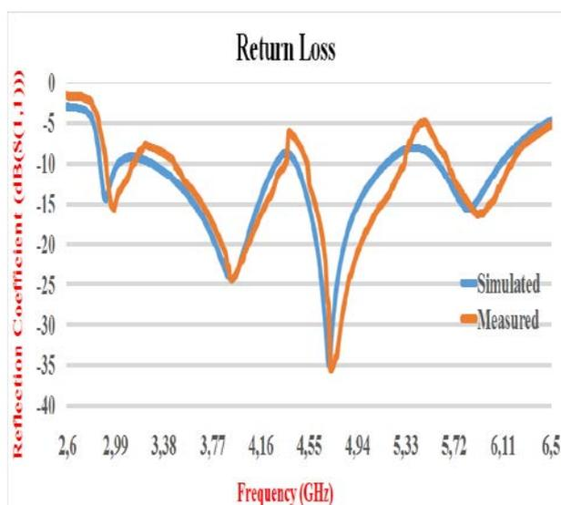
Fig. 25 Simulated vs. Measured Results
