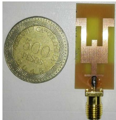
Fig. 23 Top View of DGS Microstrip Antenna
