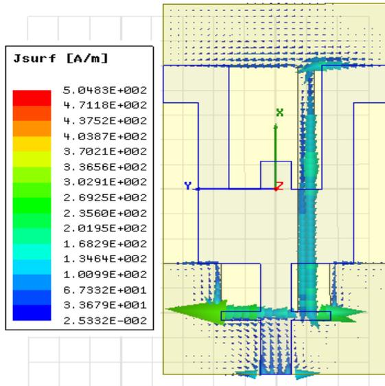
Fig. 9 Bottom View of Surface Current Density at 2.912 GHz
