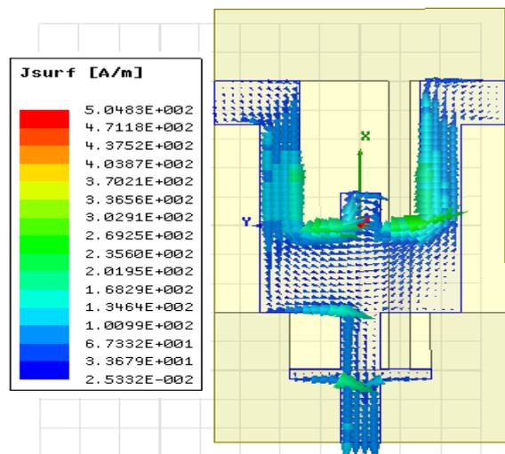
Fig. 8 Top View of Surface Current Density at 2.912 GHz
