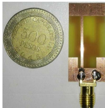
Fig. 24 Bottom View of DGS Microstrip Antenna
