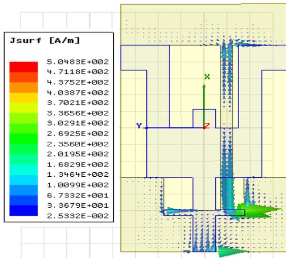
Fig. 15 Back View of Surface Current Density at 5.837 GHz
