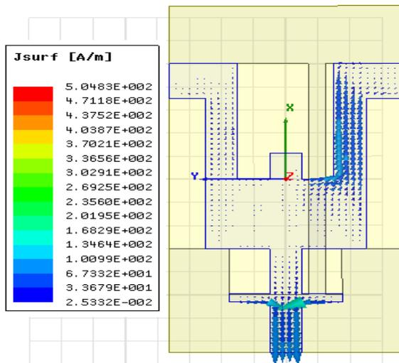
Fig. 10 Top View of Surface Current Density at 3.926 GHz
