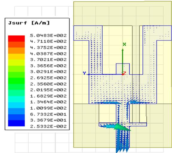
Fig. 12 Top View of Surface Current Density at 4.706 GHz
