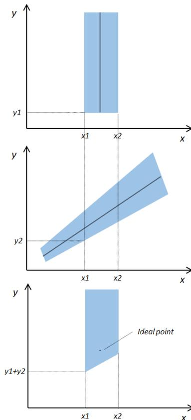
Figure 11. Convolution of Fixed Width (W) and Fixed Ratio (X) layout elements
