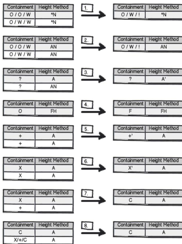
Figure 4. Consolidation of *\*N* and *AutoN* height definition methods (cases 1-3), consolidation of *FixedH (FH)* height definition method (case 4), consolidation of *Fixed Area (+)*, *Fixed Ratio (X)* and *Calc. Ratio(C)* adaptation methods (cases 5-8)
