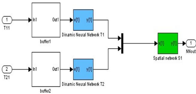
Figure 3. Connecting two dynamic networks to space network for data processing from two thermocouples
