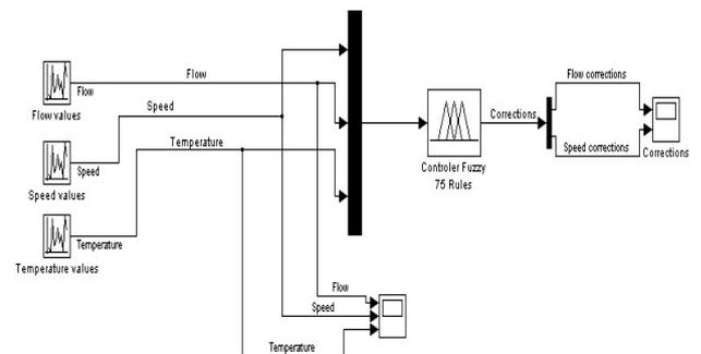
Figure 5. Simulink implementation of the fuzzy system with basic rules "1"
