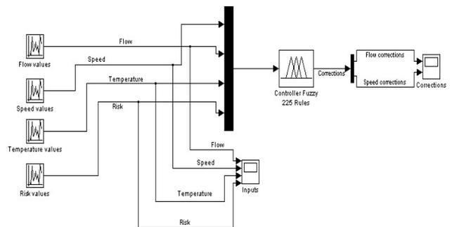
Figure 4. Implementation in Simulink to fuzzy system with basic rules “0”
