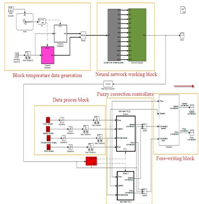
Figure 2. System implementation in Matlab-Simulink
