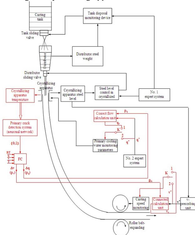
Figure 1. Control method of continuous casting process
