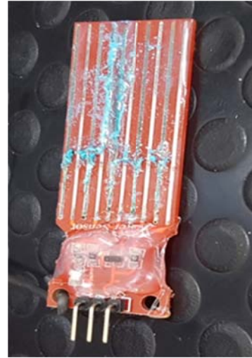
Fig. 7 Corrosion of sensor for water level
