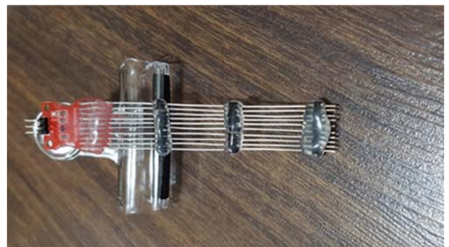
Fig. 8 The improved sensor for water level
