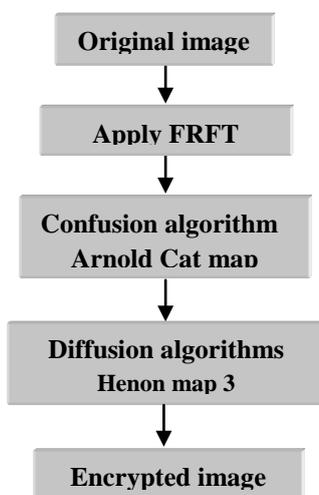
Figure 4 The block diagram of the proposed scheme 2.
