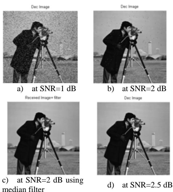
Figures (15) Reconstructing image at different SNR besides error correction code
