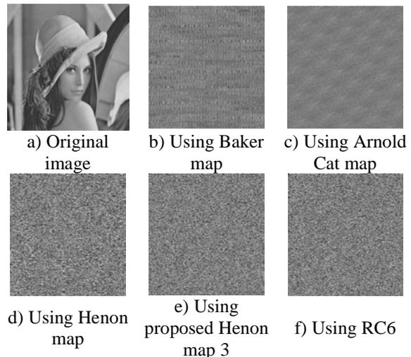
Figure (5) The encrypted image using Different chaotic Maps
