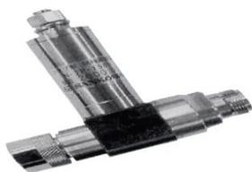
Fig.5 Appearance of  $\lambda/4$  short stub
