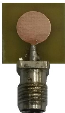
Fig. 11. Front view of the antenna built.
