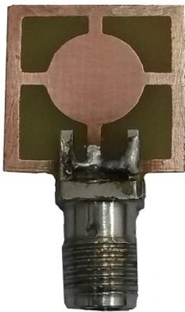
Fig. 12. Back view of the antenna built.
