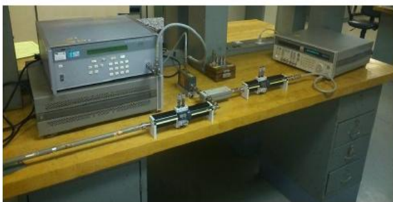
Fig. 2. Implementation of the Tuned reflectometer on Coaxial
