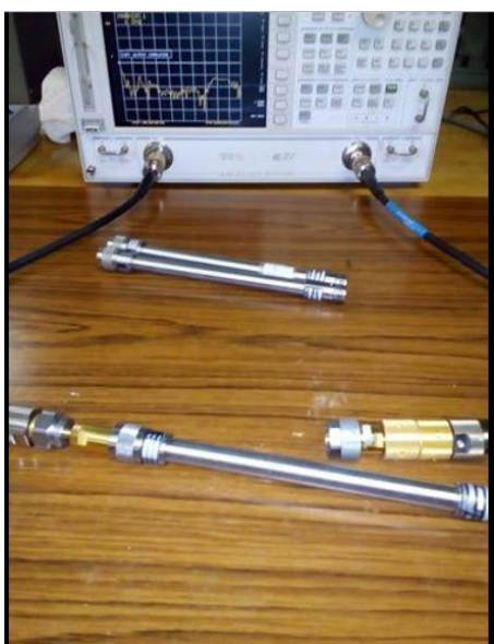
Fig. 8. Operating Mode of Measurement of reflection factor within VNA
