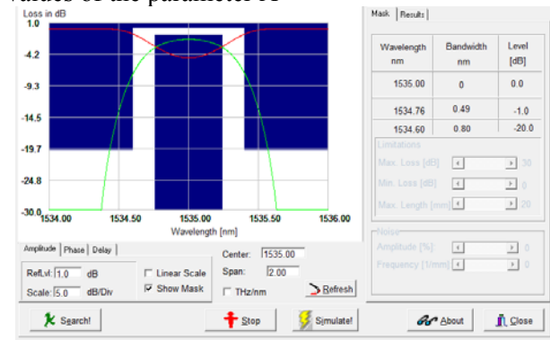
Fig. 8 Comparison of fiber Bragg gratings spectral characteristics without apodization – blue line and apodized cosine function for wsp. A = 2 – red line
