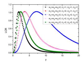
Fig.1. LCR of ratio of product of two Nakagami-*m* random processes and Nakagami-*m* random process
