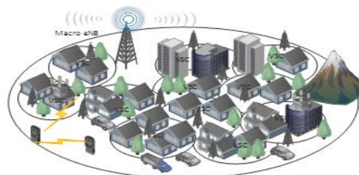
Fig. 2 Small Cells in 5G wireless system
