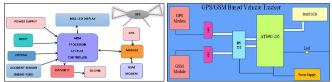
Fig. 2. (a) Automatic Vehicle Accident Detection System [7] (b) Vehicle Tracking System [9]
