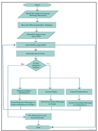
Fig. 5. Flowchart of Car Accident detection
