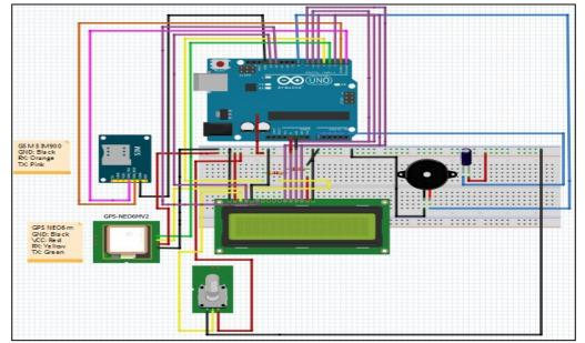
Fig. 6. Simulated diagram for the complete circuit design
