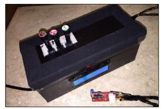
Fig. 9. Microcontroller-Based Accident Detection System
