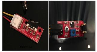
Fig. 10. The airbag sensor and the vibration sensor
