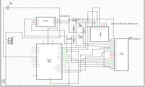
Fig. 7. Schematic diagram for the complete circuit design
