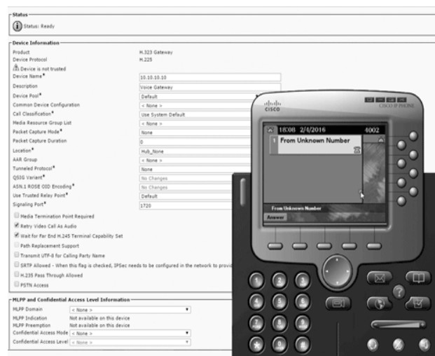
Fig.10. Explanatory scheme on showing an unknown number on the phone display in absence of a routing plan. Sources: Display Capture [12].
