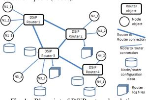
Fig. 1. Blueprint of DSiP network solution
