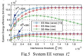
In Fig.5, we illustrate the EE versus the interference threshold  $I_p^{th}$  with/without considering sensing errors (cse/wcse) under different individual total transmit power. It can be observed that the
