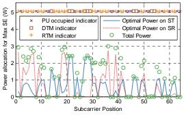
Fig.3 Power allocation on SU's each subcarrier link for maximizing SE
