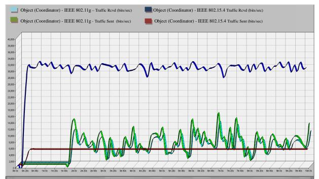
Fig. 9. Coordinator statistics -Traffic received, Traffic sent (bits/sec) comparison for both protocols
