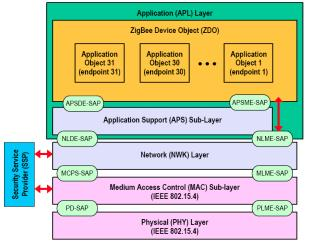
Fig. 1 ZigBee Communication Stack
