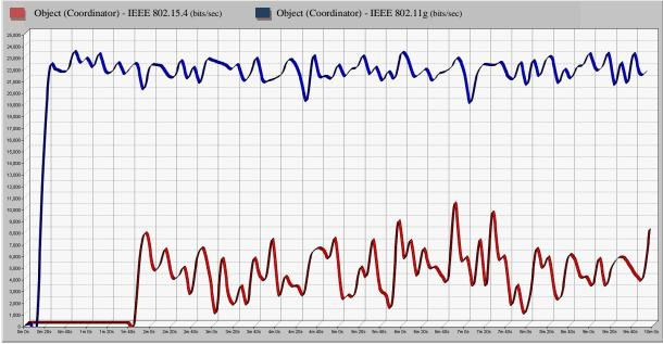
Fig. 8. Coordinator statistics – Throughput (bits/sec) comparison for both protocols
