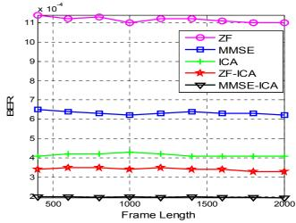
Fig. 7 shows the achieved bit-error-rates (BER) for different methods as a function of frame length (bits)
