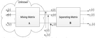
Fig. 1 General framewok for independent component analysis
