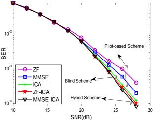
Fig.6 shows the achieved bit-error rates (BER) for the methods as a function of SNR.
