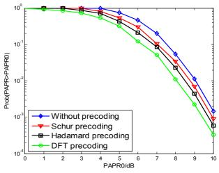
Fig.5 shows the PAPR for the different precoding methods as a function of PAPR0.
