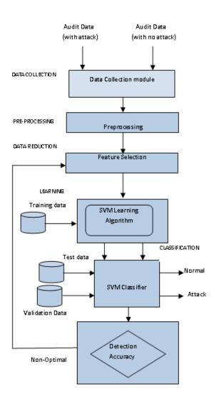
Fig.1. Architecture of the Proposed System
