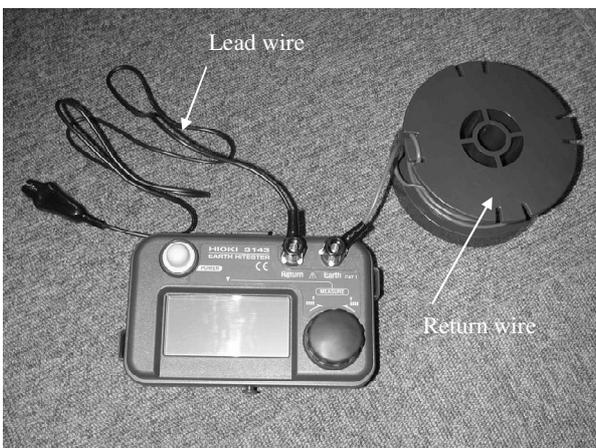
(b) A new tester and a return wire and a lead wire (rolled)
