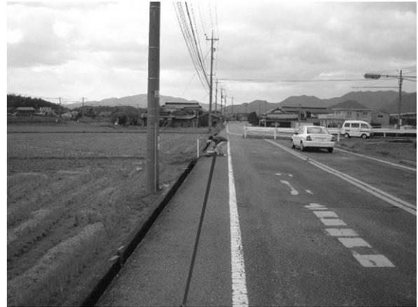
(b) A return wire is put on an asphalt road 2
