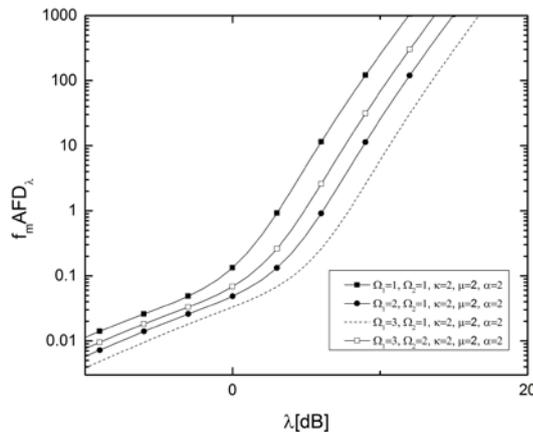
Fig.6. Normalized AFD versus SC output SIR for different parameters  $\Omega_1$  and  $\Omega_2$ , and  $\bar{a}$ ,  $k$ ,  $i=2$ .
