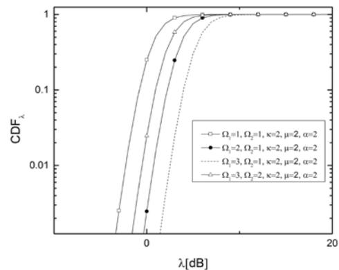
Fig.4. CDF versus SC output SIR for different parameters  $\Omega_1$  and  $\Omega_2$ , and  $\alpha, k, \mu=2$ .
