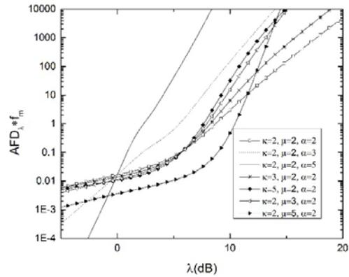
Fig.3. Normalized AFD versus SC output SIR for different parameters  $\alpha, k, \mu$  and  $\Omega_1=3, \Omega_2=1$ .
