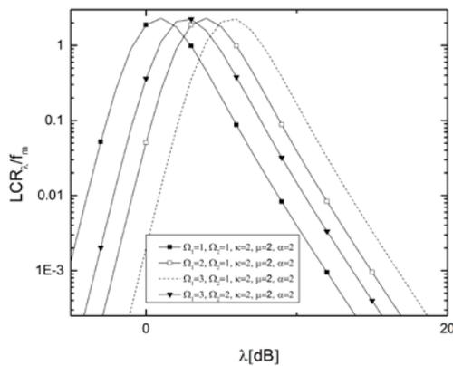
Fig.5. Normalized LCR versus SC output SIR for different parameters  $\Omega_1$  and  $\Omega_2$ , and  $\bar{a}$ ,  $k$ ,  $i=2$ .
