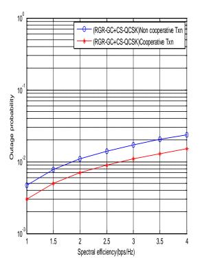
Fig.4 Outage Probability Versus Spectral Efficiency of proposed scheme in Cooperative relaying scenario
