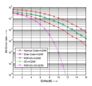
Fig. 2 BER performance comparison of the proposed Coding / modulation logic with 4-QAM
