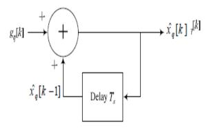
Fig.1(b) Receiver Fig.1 DPCM Technique
