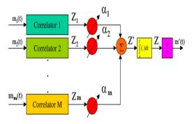
Fig. 2 Rake Receiver model data aggregation scheme
