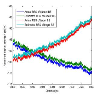
Figure 4 Comparison between Actual and Estimated received signal strengths of current and target network
