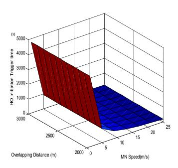
Figure 6. Handover initiation time versus Overlapping distance and velocity for proposed method
