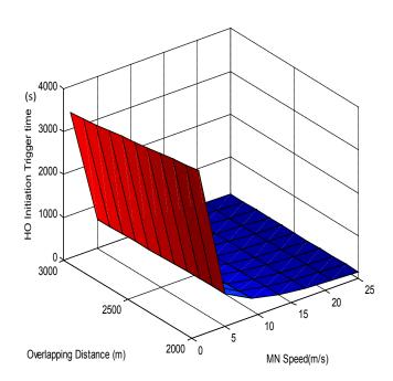
Figure 7. Handover initiation time versus Overlapping distance and velocity for conventional prediction method 1
