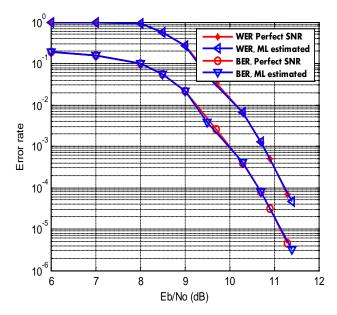
**Fig. 8** BER and WER of a rate-1/2 regular LDPC code with SNR perfectly known and estimated using ML estimation method.
