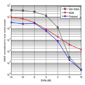
Fig. 2 NMSE of the two proposed methods as compared to the conventional SNV RXDA method.
