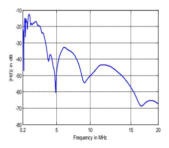
**Fig. 3** Frequency response of the 15-path reference model for PLC [22].
