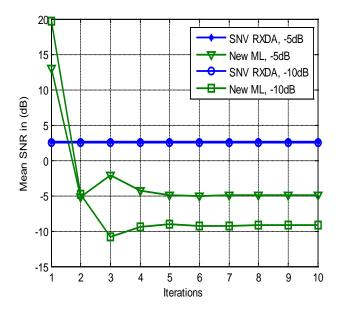
**Fig. 6** Mean estimated SNR vs. no. of iterations for ML estimation algorithm as compared to conventional SNV RXDA estimation [21] for negative SNRs.
