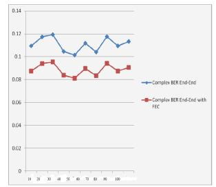
Fig. 8 Effect of length of interference on end to end BER
