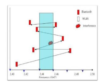
Fig. 2 Interference between Bluetooth and WLAN networks
