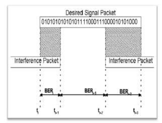
Fig. 3 Packet Collision and place of errors
