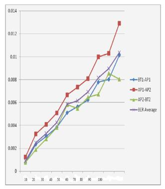
Fig. 7 Effect of length of interference in bit (x-axis) vs BER (y-axis)
