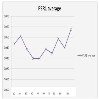
Fig. 9 Effect of length of interference in bits on Bluetooth PER 1
