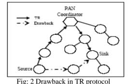
The advantage of tree routing is that it is simple and requires neither a routing table nor complexity. It only considers parent-child relationship to transmit data and ignores the neighbour nodes even if in cases in which destination address is within a single or a few hops from source node. This may cause an inefficient routing when it is routed through many hops by Zigbee tree routing algorithm.
