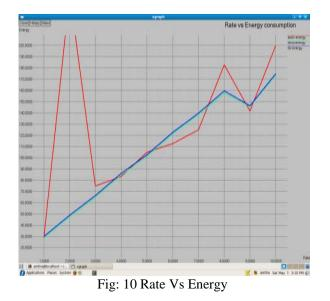
The above graph (Fig 10) illustrate the consumed energy depends on rate. If the rate increased as per the packet flow automatically the energy consumption also increased in AODV. But in our proposed CLZBRP shows the low energy level consumption than existing protocol. Because it transmits minimum overheads than AODV and TBR.
