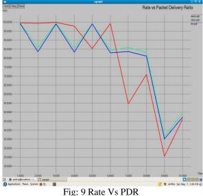
Fig 9 shows Based on the rate our CLZBRP increases the packet delivery ratio than AODV and TBR when the network size is large and the mobility is high.
