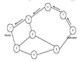
Fig. 4. The forwarding of Route Reply packet
