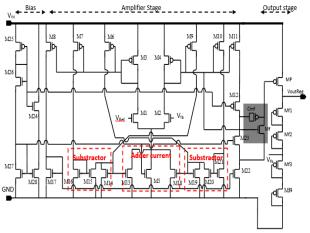
Fig 1. Conceptual schematic of the proposed LDO
