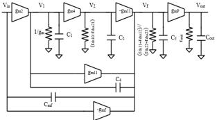
Fig 5. Small signal model of the proposed LDO
