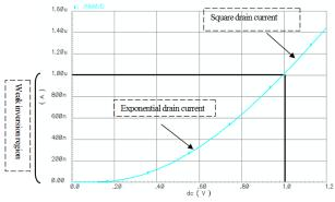
Fig 2. Characteristics of the transistor in the weak inversion region
