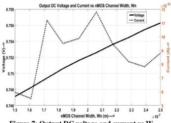
Figure 7: Output DC voltage and current vs W<sub>n</sub>
