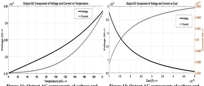
Figure 11: Output AC components of voltage and current vs Temperature
