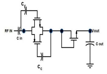
Figure 2: Proposed 3-transitor rectifier with threshold voltage compensation
