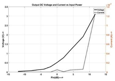
Figure 14: Output DC voltage and current vs  $P_{in}$  As the PCE of the circuit is the major and significant performance parameter, it is evaluated and presented in Fig. 15. T he PCE obtained are 90% and 85% at 2db and -2db resp ectively. For higher input power, power gain is also observed. This clearly shows the efficacy of the design particularly at low input power applications.
