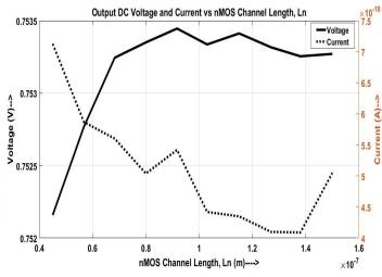
Figure 6: Output DC voltage and current vs L<sub>n</sub>
