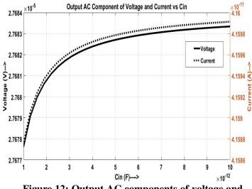
Figure 12: Output AC components of voltage and current vs  $C_{\rm in}$
