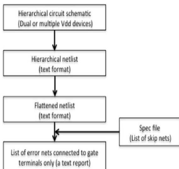
Fig. 4 Flow to Detect Floating Gate Faults.
