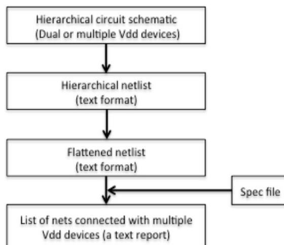
Fig. 3 Flow to Detect HV/LV Connection Faults.
