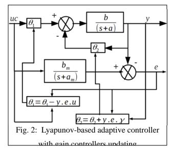
We fixed the value  $\gamma$  as 0.3. The parameters of the plant is a=0.9 and b=0.1. The parameters of the reference model is am=1 and bm=0.2 It was applied a unit step as input. At each sample time the controllers gains are updating according to Fig. 2.
