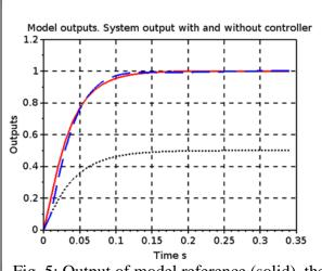
Fig. 5: Output of model reference (solid) the plant with controller (dash) and without
