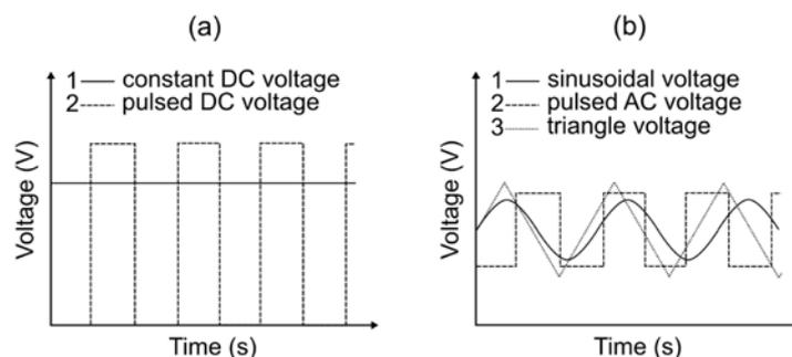
Fig. 6. DC and AC actuating signals for the electric field modifier electrode: a) Constant DC voltage (a.1) and pulsed DC voltage (a.2); b) AC actuating signals with variable frequencies and amplitudes: b.1) sinusoidal voltage; b.2) pulsed voltage; b.3) triangle voltage.
