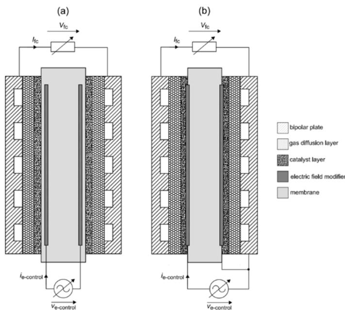
Fig. 5. Possible profiles of PEM fuel cells with two electric field modifiers (EFM) in or at the membrane and examples of electric circuits with a variable AC voltage source: a) The potential of the EFM is independent of the fuel cell electrode potentials; b) The potential of the EFM is dependent on the potential of the anode or cathode.
