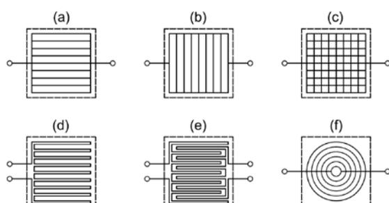
Fig. 3. Simplified drawings of possible single and double layer electric field modifier (EFM) electrodes: a) horizontal grid; b) vertical grid; c) meshed grid; d) single controlled comb-shaped structure; e) double controlled comb-shaped structure; f) circle pattern.
