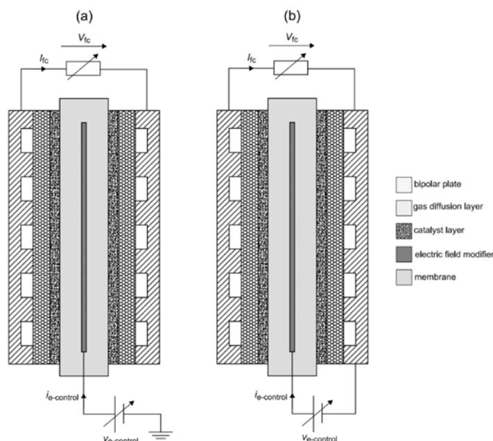
Fig. 4. Possible profiles of PEM fuel cells with a single electric field modifier (EFM) in the membrane and examples of electric circuits with a variable DC voltage source: a) The potential of the EFM is independent of the fuel cell electrode potentials; b) The potential of the EFM is dependent on the potential of the anode or cathode.
