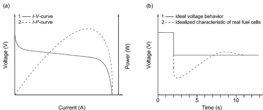
Fig. 1. a) Characteristic  $I$ - $V$ -curve (a.1) and  $I$ - $P$ -curve (a.2) of a fuel cell; b) Dynamic fuel cell voltage characteristics after a positive current step at  $t = 2$  s: b.1) ideal voltage response; b.2) idealized dynamic voltage behaviour of actual fuel cells.
