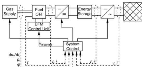
Fig. 7. New simple power electronics subsystem with an electric field modifier (EFM) control unit, own representation and extension according to [17]: reactant flow rate  $dm/dt$ , reactant partial pressures  $p$ , reactant relative humidity  $\phi$ , operating temperature  $T$ , fuel cell voltage  $v$ , fuel cell current  $i$ , and internal controlling voltage  $v_{e-control}$ .
