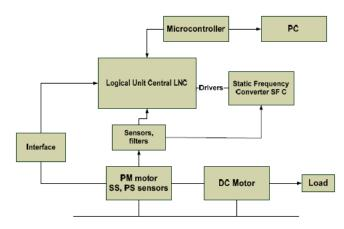
Fig. 2 General diagram of the test bench
