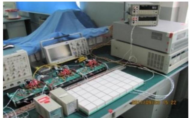
Fig.10 Experimental platform of three-module NIWC system
