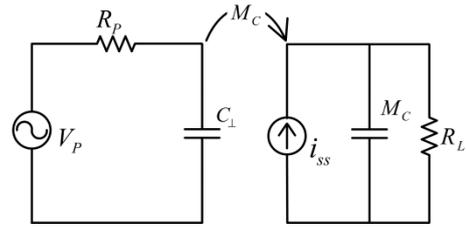
Fig.8. Equivalent circuit model of meander-type coupled structure
