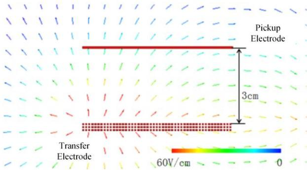
Fig.5. Electricfield distribution of meander-type coupled structure
