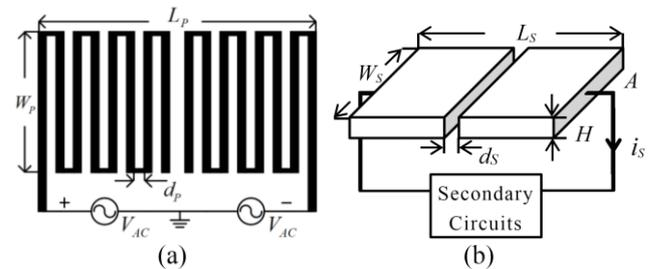
Fig. 4. Structure of meander-type transmitting and receiving electrodes
