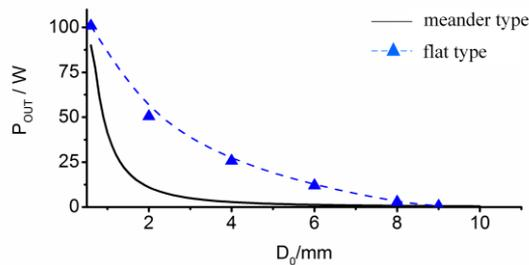
Fig.10. Transfer capability curves of meander-type CCPT system varying with D
