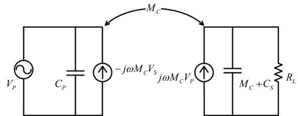
Fig.9. Equivalent circuit smodel of flat-type coupled structure
