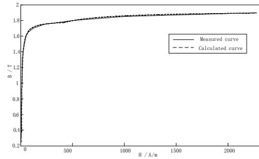
Fig.6 The magnetization curve of Measured and calculated
