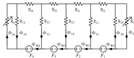
Fig.3 Magnetic circuit model of CRT
