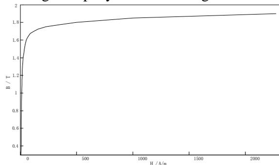
Fig.5 Magnetization curve of grain-oriented magnetic steel sheet
