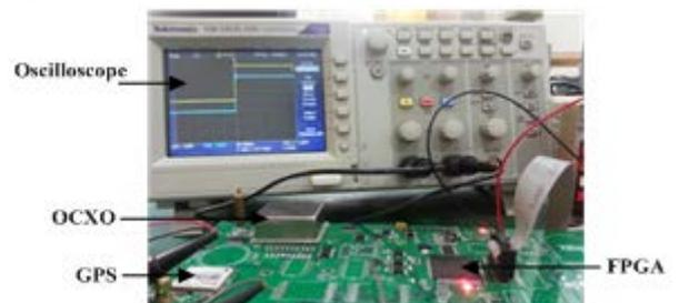
Fig.11 The debugging diagram of prototype for GPS and OCXO timing
