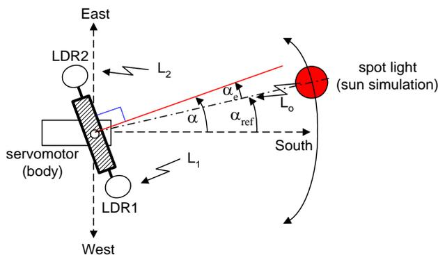
Figure 5: Reference angles (top view)
