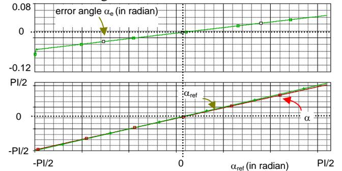
Figure 21: Closed loop transient response and residual static error  $\alpha_e$
