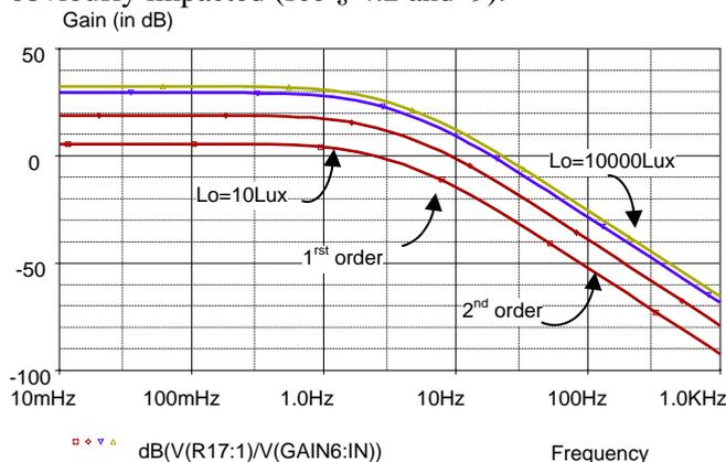
Figure 20: Open loop simulation (AC)
