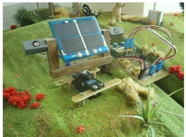
Figure 26: small scale solar tracking system installation
