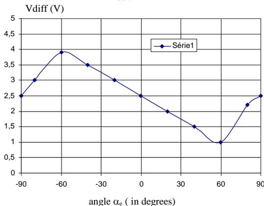
Figure 28: Sensor  $V_{diff}$  vs. angle  $\alpha_e$  (in degrees)
