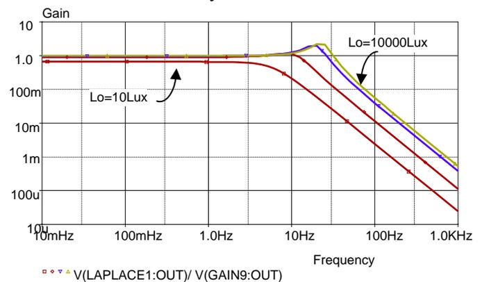
Figure 22: Closed loop AC response
