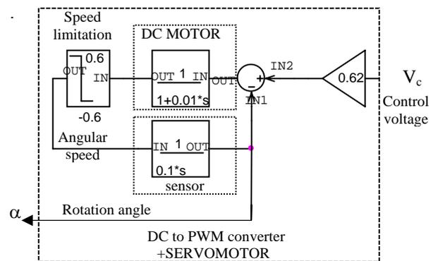
Figure 15: DC/PMW and Servo motor SPICE modelling
