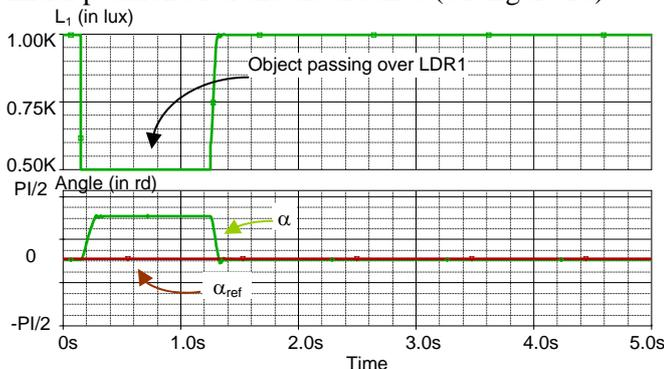
Figure 24: Closed loop transient response to a disturbance on D input.
