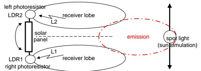
Figure 3: Solar panel alignment
