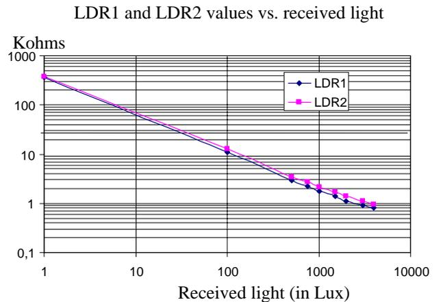
Figure 10: Static LDR characterisation
