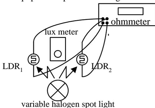
Figure 9: LDR static characterisation test bench
