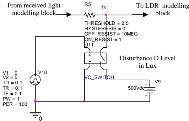
Figure 16: Disturbance input modelling
