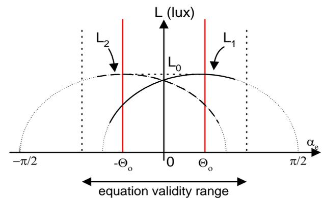
Figure 7: Received light  $L_1$  and  $L_2$  vs. angle  $\alpha_e$
