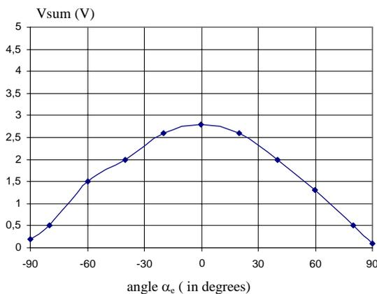
Figure 29: Sensor scaled voltage  $V_{sum}$ , vs. angle  $\alpha_e$  (in degrees)
