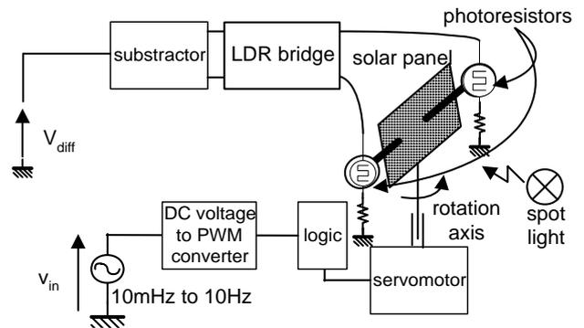
Figure 30: Open loop dynamic characterisation schematic
