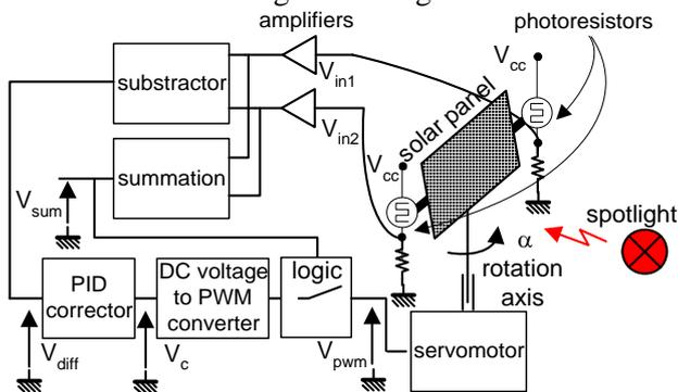
Figure 2: Sun tracking system block diagram
