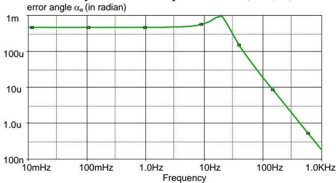
Figure 23: Closed loop response to fluctuation of source intensity (I input).
