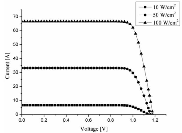
Fig.2 I-V characteristics of GaAs concentrator cells
