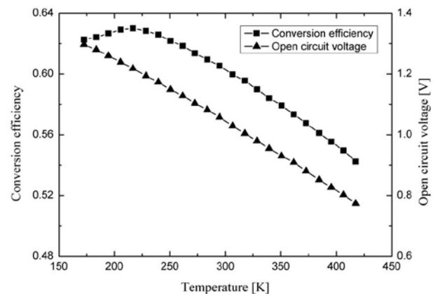
Fig.5 Variation of  $\eta$  and  $V_{oc}$  with temperature for GaAs cells
