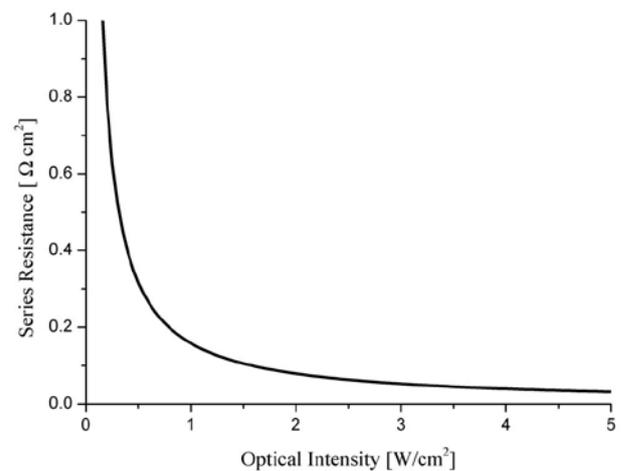
Fig.3 Calculated series resistance of GaAs concentrator cells
