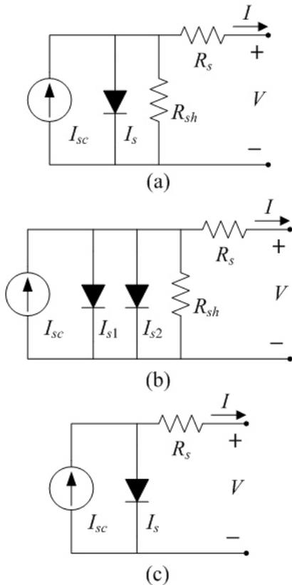
Fig.1 PV cells equivalent circuit models: (a) single-diode model, (b) two-diode model, (c) simplified equivalent model
