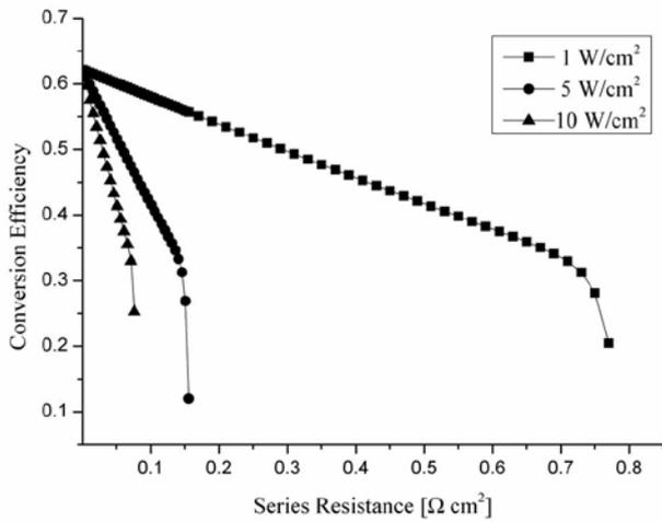
Fig.4 Conversion efficiency as a function of series resistance
