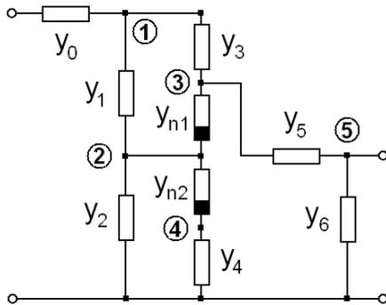
Fig. 7. Five-node nonlinear passive network.
