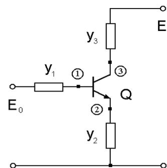
Fig. 9. One-stage transistor amplifier.
