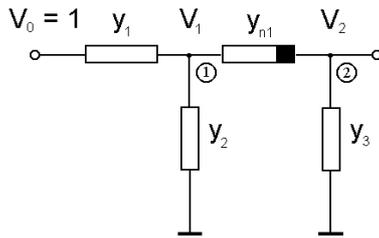
Fig. 1. Two-node nonlinear passive network.
