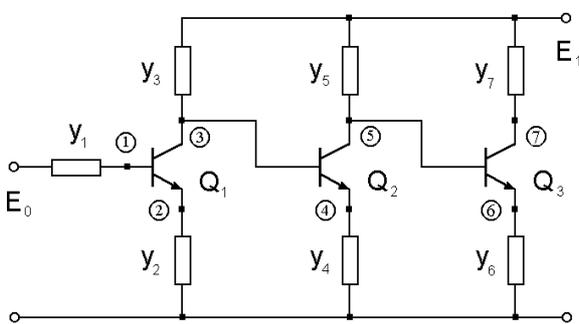
Fig. 13. Three-stage transistor amplifier
