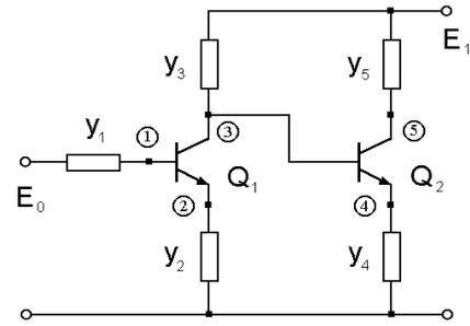
Fig. 11. Two-stage transistor amplifier.
