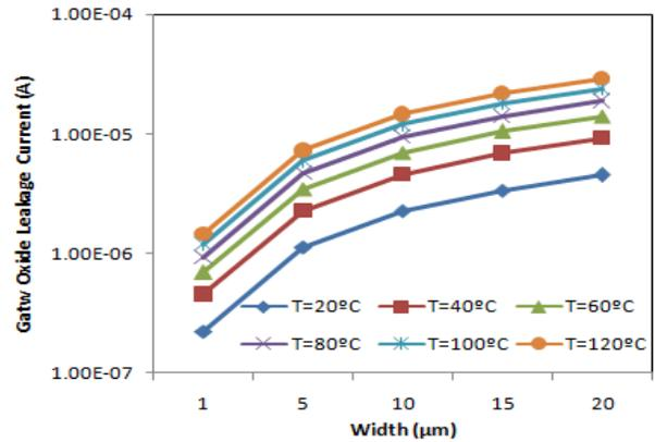
Fig 3. Variation of the gate-oxide leakage current with temperature and width of transistor.
