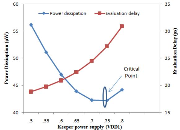
Fig 8. Evaluation delay and power dissipation of HVT domino XNOR gate with dual power supply.
