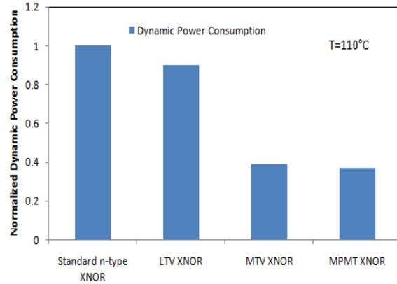
**Fig 12.** Comparison of the dynamic power consumption with four techniques at 110°C. Dynamic power consumption is normalized by standard n-type XNOR for each circuit.
