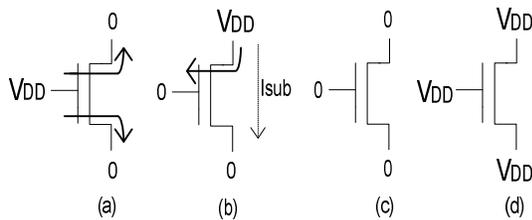
Fig 1. (a) Maximum gate-oxide leakage current state, (b) Maximum subthreshold leakage current state, (c) and (d) condition to avoid both subthreshold and gate oxide leakage current .
