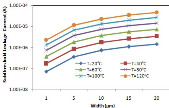
Fig 2. Variation of the subthreshold leakage current with temperature and width of transistor.
