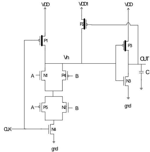
Fig 7. MTV Domino XNOR gate with dual power supply.
