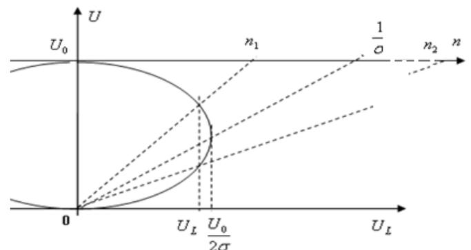
Fig.8. Geometrical model of the regulated characteristic of a boost converter
