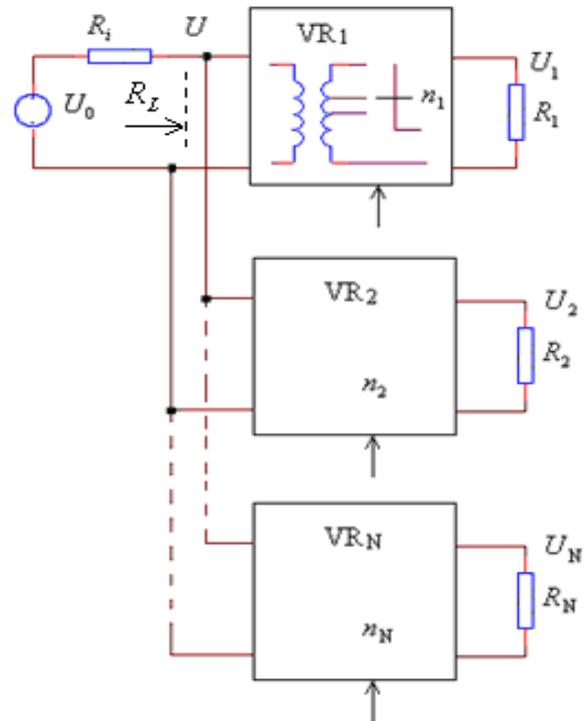
Fig.1. Power supply system with two voltage regulators  $VR_1, VR_2$  and loads  $R_1, R_2$
