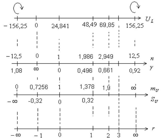
Fig.11. Example of regime change and conformity of points of the axes  $U_L, n, \gamma$  of the boost converter
