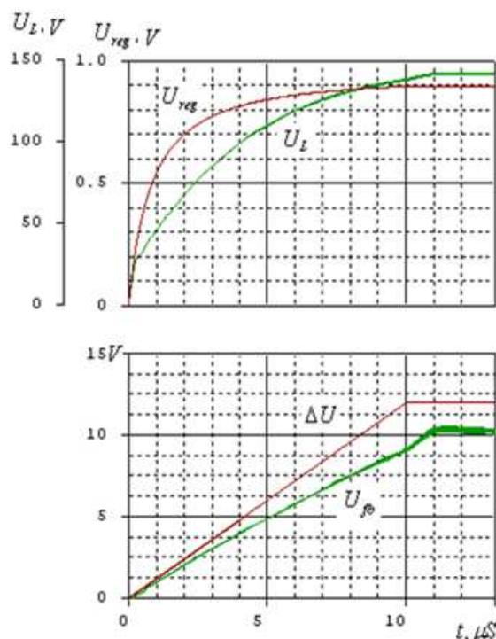
Fig. 14. Results of modeling of the boost converter with the linearized regulated characteristic.
