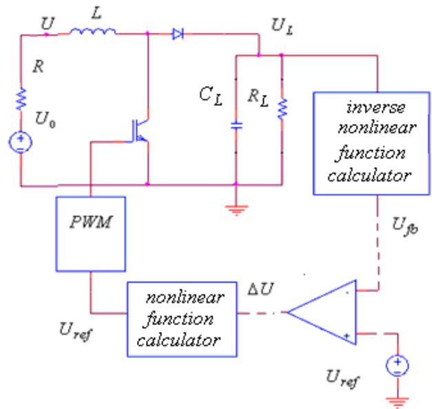
Fig.7. Boost voltage converter with linearization function calculators of control voltage  $\Delta U$  and feedback voltage  $U_{fb}$
