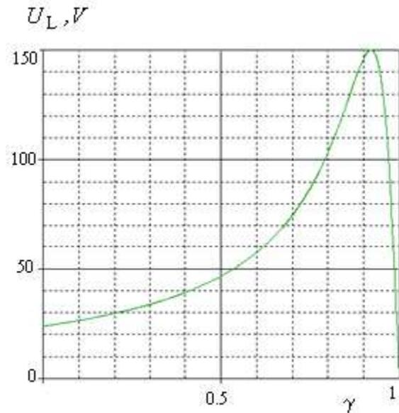
Fig.10. Regulated characteristic of the boost converter
