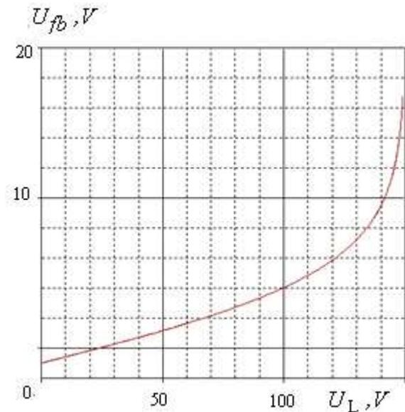
Fig.13. Inverse nonlinear function calculator characteristic
