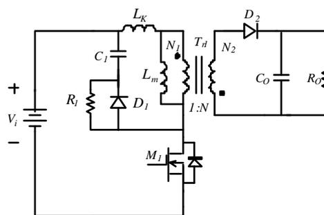
Fig. 1. Schematic diagram of flyback converter with conventional RCD snubber.
