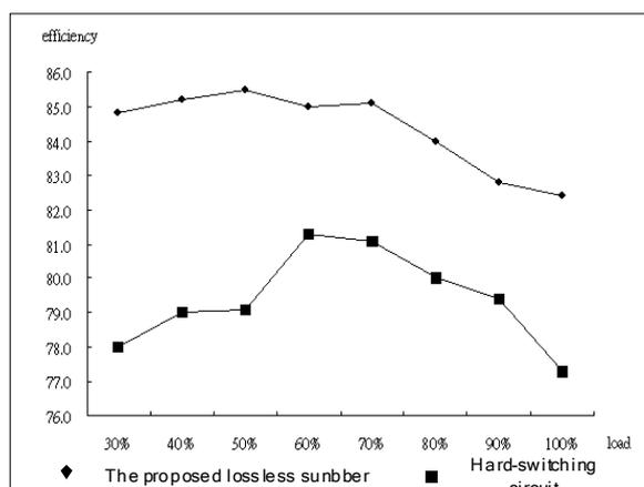
Fig. 11. Comparison of efficiency between the proposed auxiliary power supply under hard-switching and with the proposed lossless snubber from light load to heavy load.
