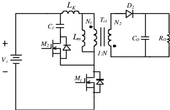
Fig. 3. Schematic diagram of flyback converter with conventional active clamp circuit.
