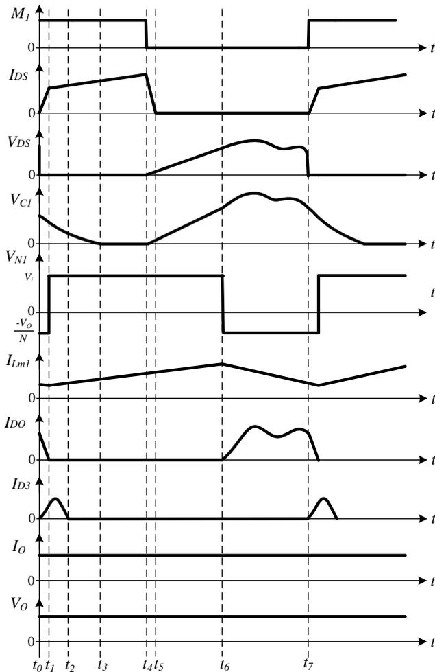
Fig. 8. Key waveforms of the proposed converter.
