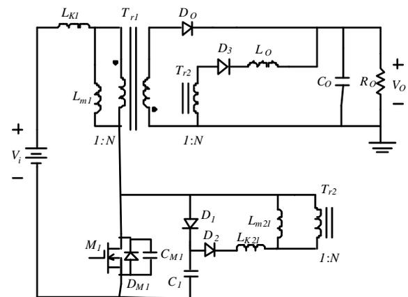
Fig. 5. Schematic diagram of flyback converter with the proposed lossless snubber.
