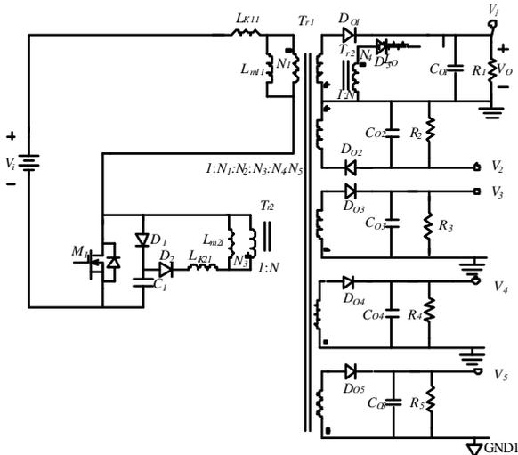
Fig. 6. Schematic diagram of the proposed auxiliary power supply with five sets of output voltages.
