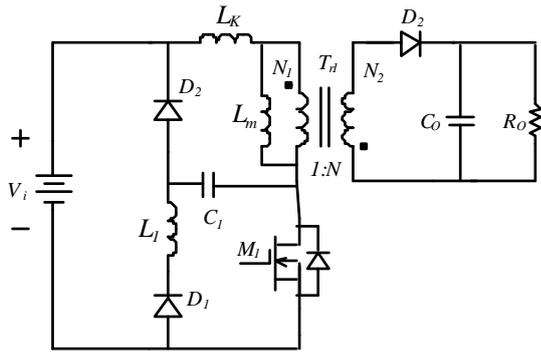
Fig. 2. Schematic diagram of flyback converter with lossless LCD snubber.
