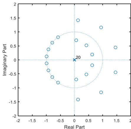
Fig. 11 – Zero-pole plot of the LPF
