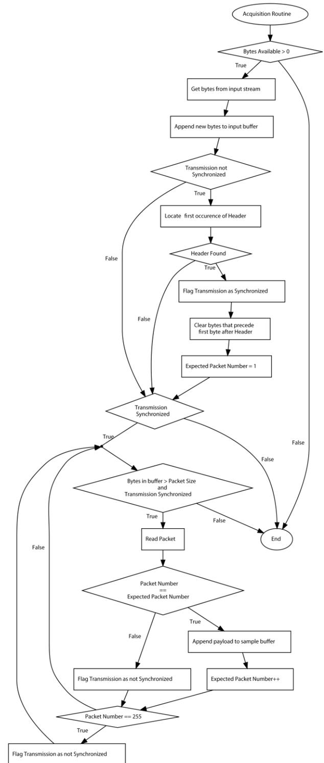
Fig. 7 – Acquisition routine’s flowchart
