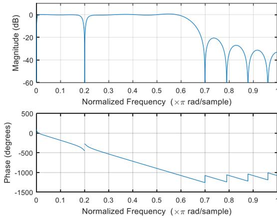
Fig. 10 - Normalized frequency response of the high-pass, low-pass and notch filters' cascade
