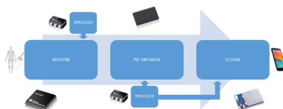
Fig. 1 – Bluetooth<sup>®</sup> electrocardiograph block diagram
