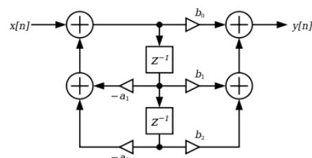
Fig. 9 – Direct Form II flow graph of a 2nd-order filter.
